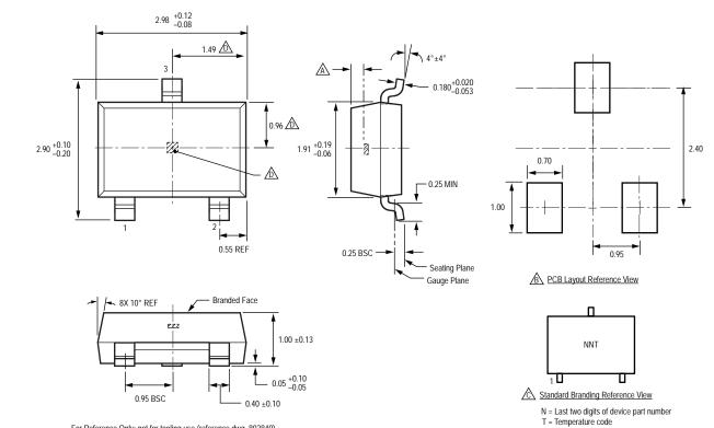
For Reference Only; not for tooling use (reference dwg. 802840) Dimensions in millimeters
